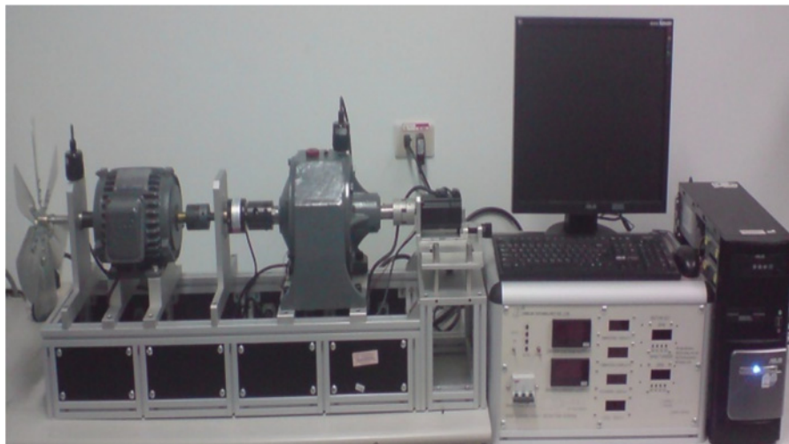
Fig. 2 Experiment platform for wind power generation system of this paper
